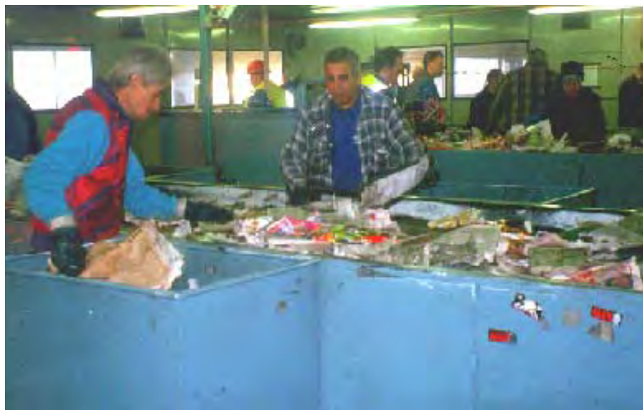
Plate 5.3 Sorting Conveyors within a Materials Recovery Facility (MRF)
